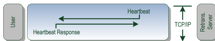
Figure 7: Retransmission Server Heartbeat Message
